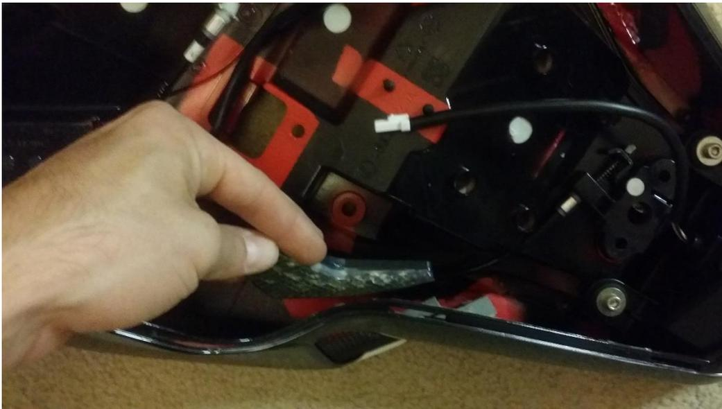
5. The light should now be held in place loosely. Look at the vent from the outside and make sure the light is centered in the vent mesh, adjust if necessary.
