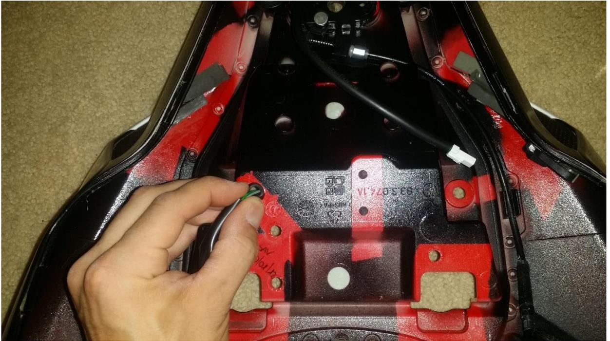
11. Feed the supplied wire harness through the hole, and then through the rubber grommet. Be gentle when feeding the wire harness through the grommet as it does take some force. Once the wire harness is through, reinsert the grommet back into the hole.
