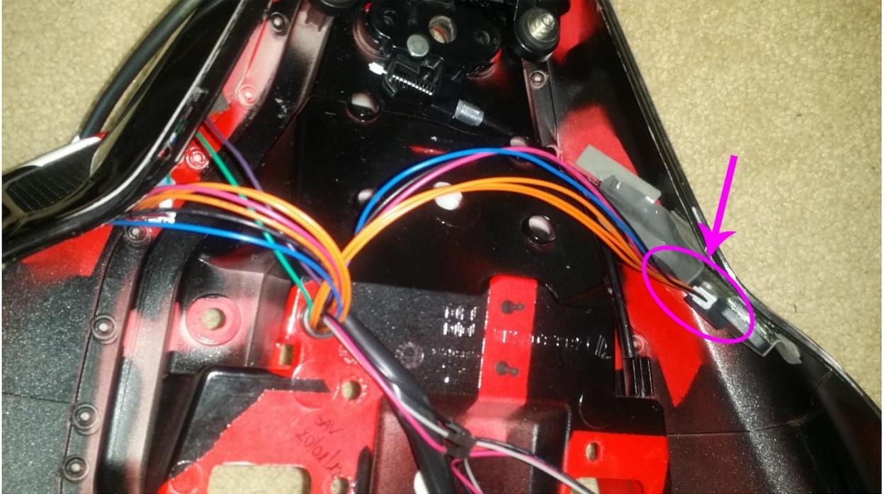
14. Plug in the brake light connector from your brake light into the harness. (If you have an integrated tail light and Brakers Integrated wire harness, you will have 2 additional plugs for the turn signal wires coming out of your tail light).
