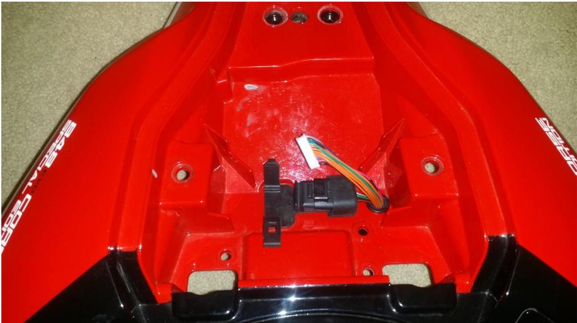
12. Plug the connector on the wire harness into the Control Unit, then remove the protective backing from the adhesive strip on the back of the control unit, and stick it in the trunk wherever you prefer.
