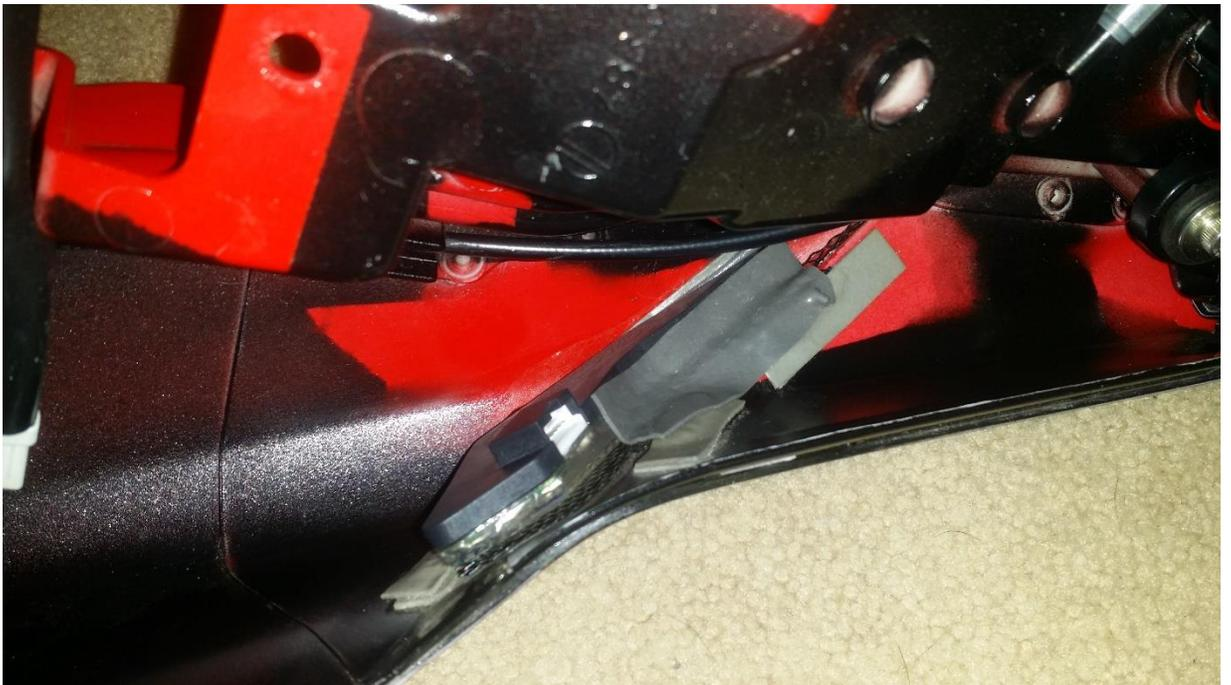
(Make sure you jam the tape into all the gaps between the light and the tail fairing. This will ensure the strongest bond. You want the adhesive to make contact with as much surface area on the tail section as possible.)
