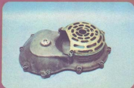
Running with a dry clutch means a special mag. alloy casting for the primary drive.
