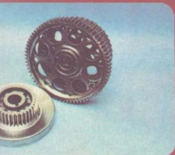
Flywheel is lightened and polished: drive gears are special factory jobs.
