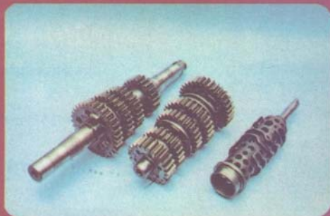
A close ratio five speed gear cluster is fitted, many of the gears are drilled for lightness.
