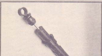
20 The rear shock absorbers are Girling gas units, the latest road type with pre-load adjusters.
