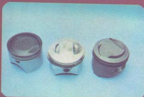
Teflon coated 11:1 piston (right), standard (centre) and endurance 8:1 (left).
