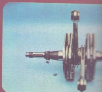
Due to the heavier crankpin and pin has to be re-balanced.
