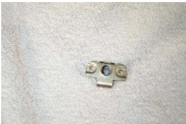
Modified rivet plate to follow the contour of the front of the reservoir.
