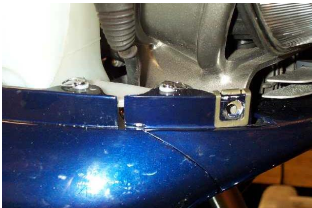
Side view of the two long Dzus fasteners connecting the front Ram Air and upper right fairing panels to the reservoir. Notice the three nylon washers to take some of the slack.
