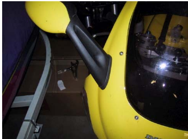
Mirror mounted on the bike with Dzus fasteners. (Wolfie's bike)
