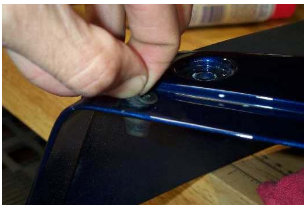
Peeling off the front face of the wellnut from fairing where it was pressed to the surface.
