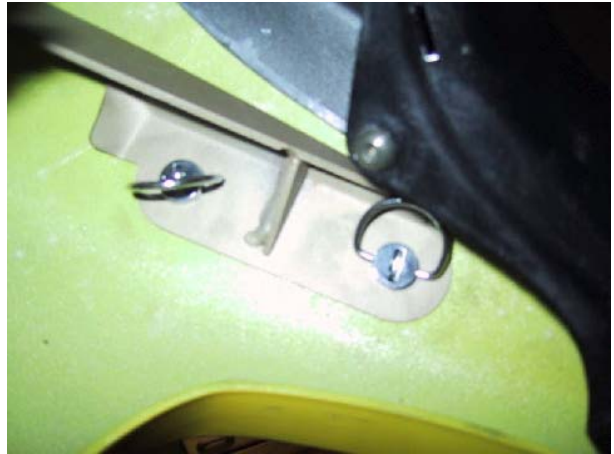
6mm Dzus fasteners holding the mirror in place. (Wolfie's bike)
