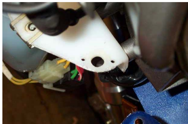
Extra holes drilled on the reservoir for mounting the rivet plate.
