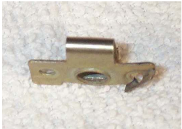
The bent piece was grounded using a bench grinder to provide a ledge for better mounting on the left frame mounting plate.
