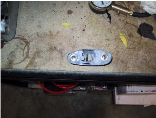
Receptacles JB Welded into the mirror base. (Wolfie's bike)
