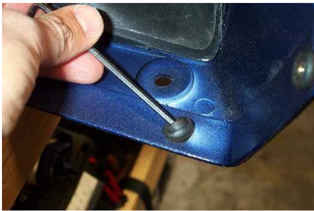
Using an Allen wrench to decompress the wellnut from the backside.
