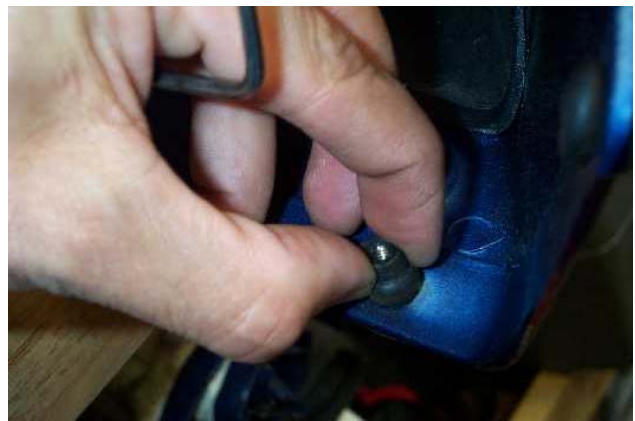
Squeezing the wellnut to decompress the rubber and making it narrower and easier to hold.
