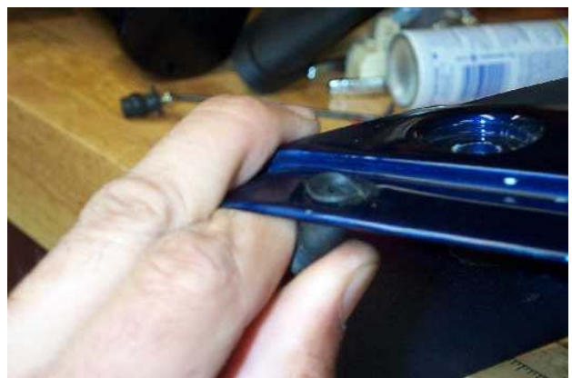
Holding the rubber with two fingers and pulling from the rear to remove the wellnut.
