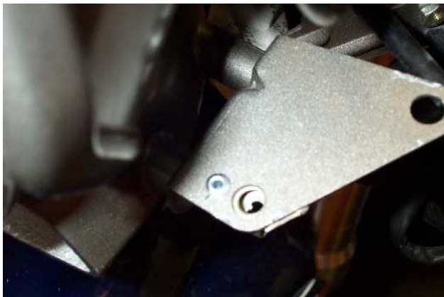
The modified rivet plate after it was riveted to the left frame mount. Notice the edge of the rivet plate holding the mounting plate.
