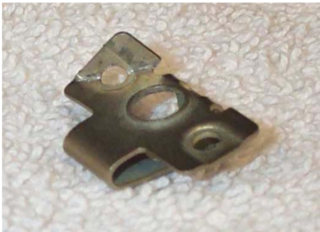
After marking a rivet plate the side of the plate was bent to follow the contour of the frame mounting plate.
