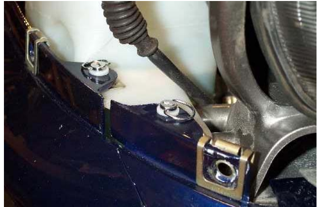
Two long Dzus fasteners connecting the front Ram Air and upper right fairing panels to the reservoir. Notice the three nylon washers to take some of the slack.
