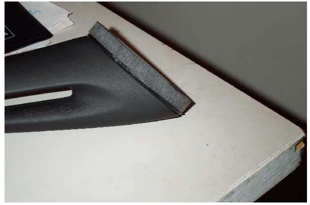
Mirror spacer mounted side view. As you can see the holding bolts are not visible from the side.
