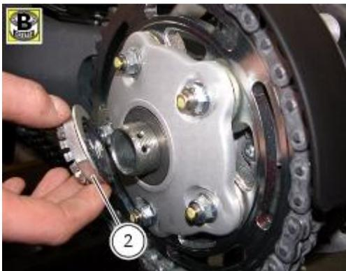
Install the safety clip (1), positioning it on the nut (2) as shown in the figure.
