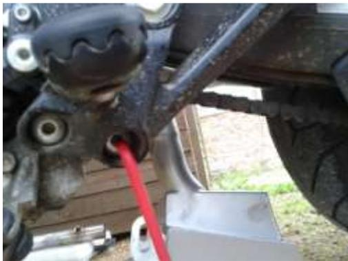
You will need a strong 8mm hex-key to undo the foot-rest assembly bolts. BEWARE!! The kick-stand is attached to the front bolt on this side so always undo these bolts with the bike on a paddock stand or leaned on something! I suggest you do one side at a time.
