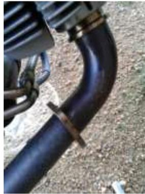
Undo manifold bolts – and keep studs/nuts for reassembly
