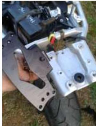
The disassembly of the tail is easily done – just ensure to unplug the registration plate light and snip off the connector to use with an aftermarket LED version.
