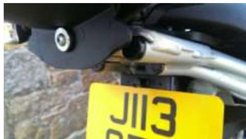
The registration plate was mounted by drilling a hole through the rear-light mounting plate (top right) and the bolting through an aftermarket 'miniature' reg-plate mount. I used a reg-plate white LED 'bolt' to mount the plate – hence a neat mounting and illumination solution. I finished off with 19mm tube plugs in the
