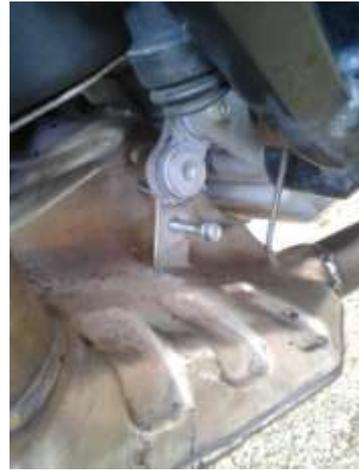
Remove the brake pedal with one bolt (the pin on the left just slips out of the rubber boot) – this allows access to the old exhaust mount. Keep all bolts!
