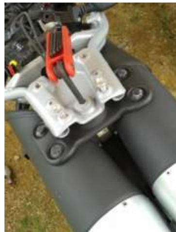
Exhaust clamp removal left (you may wish to retain it to fit the Exbox), and removal of the rear exhaust mounting bolt.
