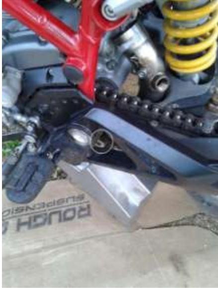
With the metal plates in position you see the 'droop' mounting hole –kick-stand side (pic1) and on the brake side (pic2) – both circled for clarity
