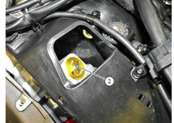
Rotate clockwise (HARD) to increase the hydraulic damping or counter clockwise (SOFT) to decrease it.
