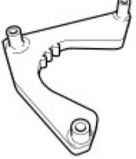
A technical drawing of a TDC control tool, which is a curved metal bracket with a central notch and two mounting points at the ends. |
