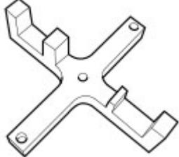
A technical drawing of a camshaft locking tool, which is a cross-shaped metal bracket with four arms and a central hole.             |
