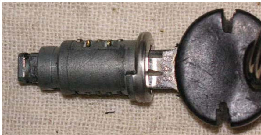
Figure 9. Right key inserted causing all the sliding plates to be retracted into the tumbler.
