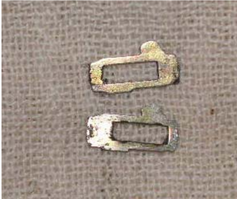
Figure 4. This picture shows two different sliding plates. Note the position of the slots in the plates with respect to the end of the plates.
