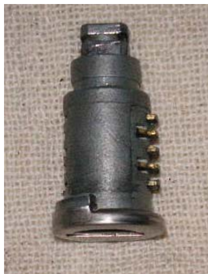
Figure 1. This is how the tumbler looks with the key removed. You can see all the sliding plates sticking out the side of the tumbler.
