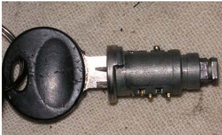
Figure 3. When the wrong key is inserted into the tumbler, one or more sliding plates will stick out of the side of the tumbler into the groove in the barrel, preventing it tumbler to rotate inside the barrel. This will not allow the latch to open.
