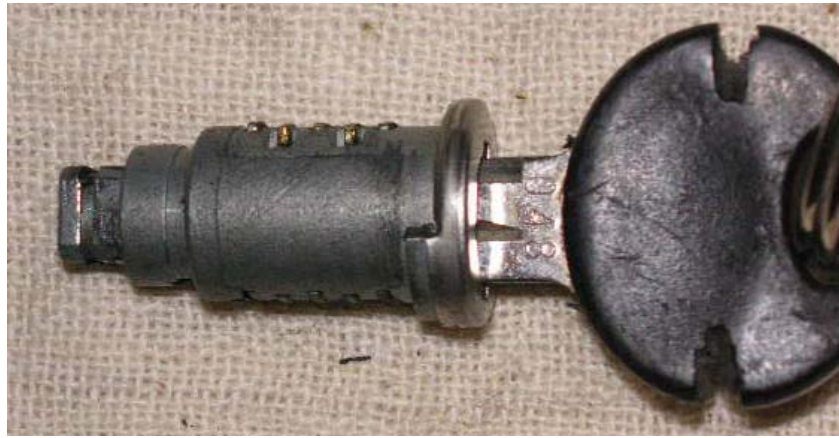
Figure 2. When the right key is inserted into the tumbler, all the sliding plates are pulled into the tumbler, allowing it to rotate inside the barrel.
