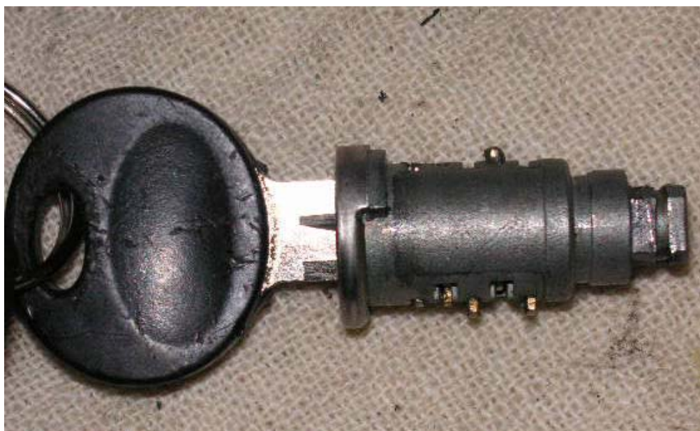
Figure 10. Wrong key inserted. Three of the sliding plates are still sticking out of the side of the tumbler.
