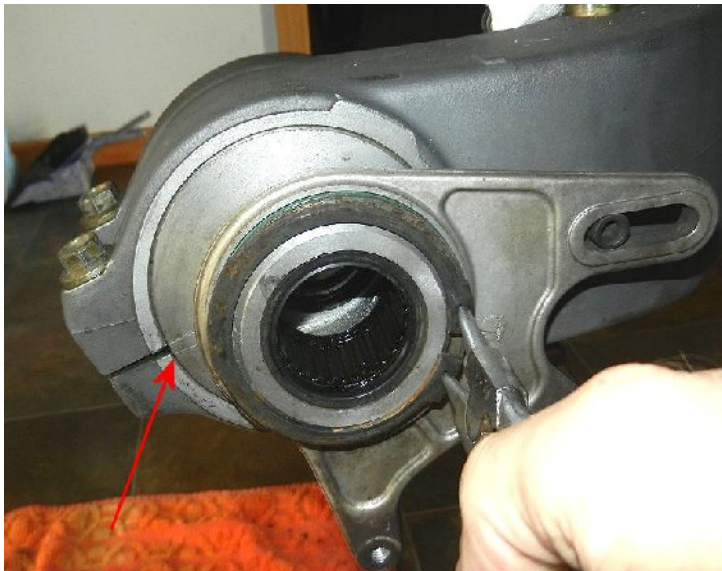
Removing the Caliper arm circlip.
