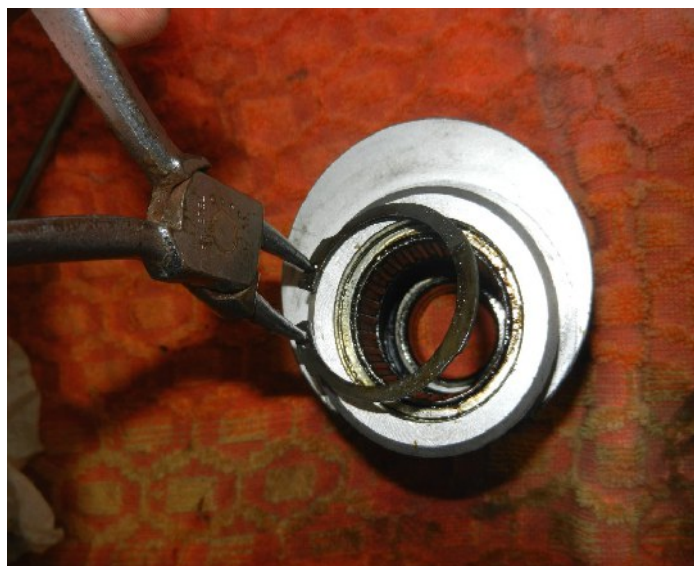
Removing the circlip from the needle roller bearing side of the hub
