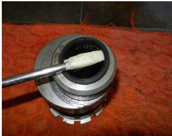
Levering the seal out with a large screwdriver
