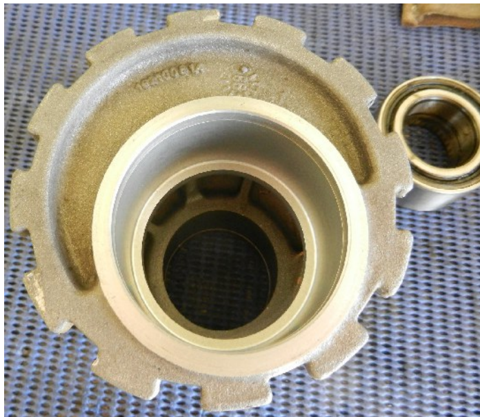
Repeat on the needle bearing side then degrease and clean the hub
