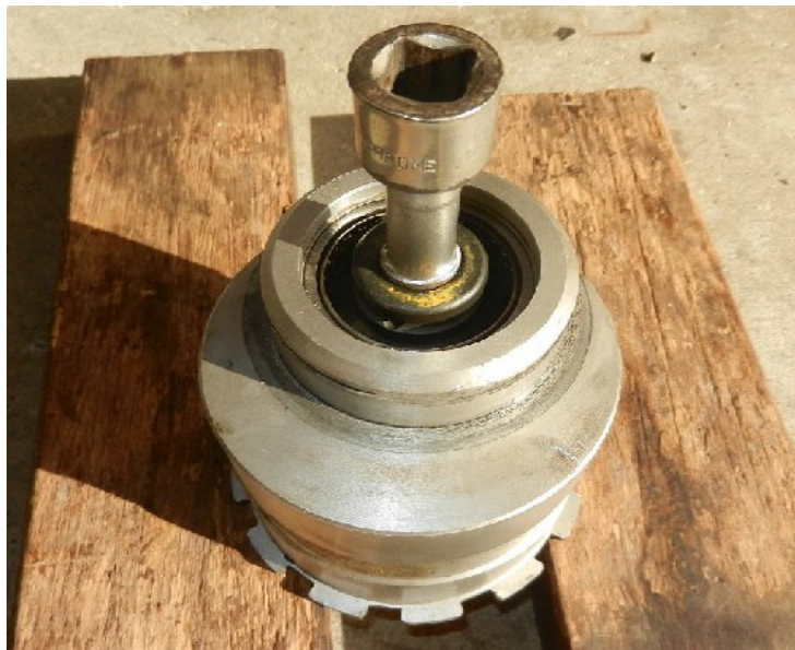
Inserting a suitable dolly to push the ball bearing out
