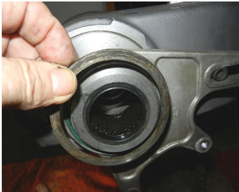
Removing the steel washer, there is one each side of the arm
