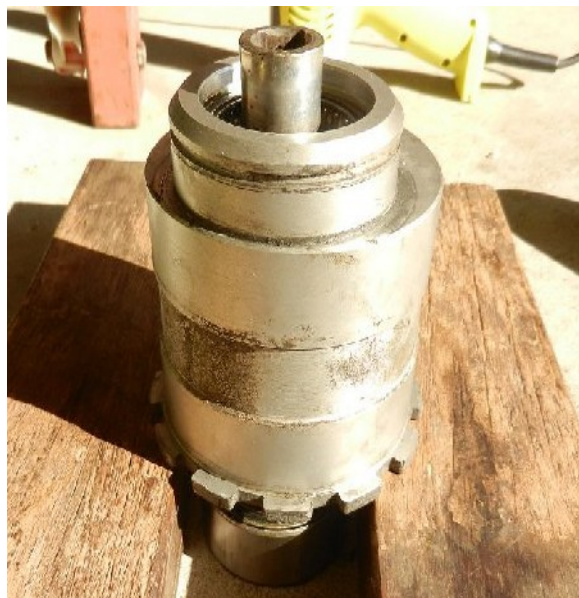
Inserting a suitable dolly to push the ball bearing out
