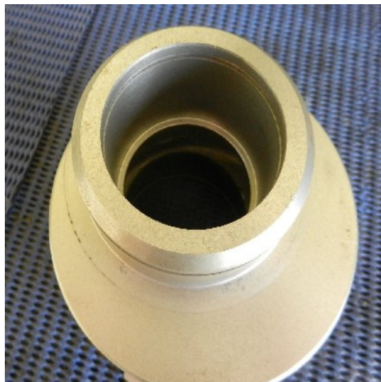
Make sure you thoroughly clean the circlip grooves out
