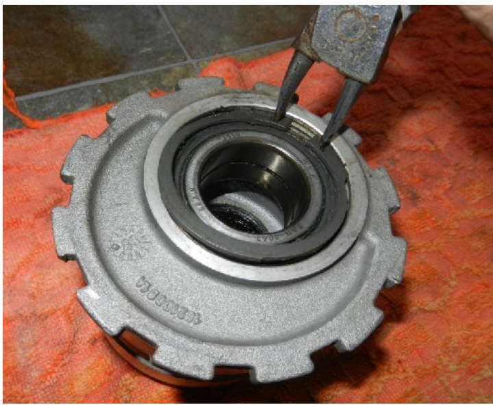
Removing the circlip from the ball bearing side
