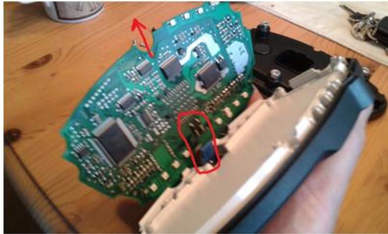
6. Mount the USB Eeprom programmer in the USB port. The pins are numbered, pin number 1 (red) is top right.
