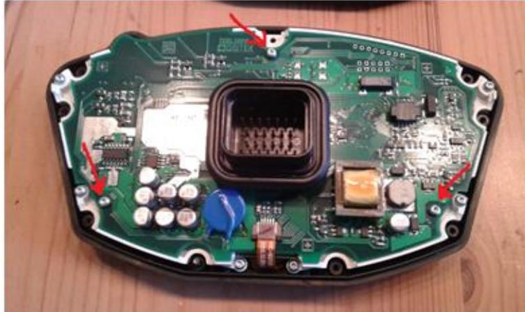
5. Lift the PCB carefully and disconnect the power cable to the PCB (just slide it off).
