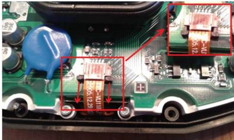
4. Unscrew the three hex screws on the PCB.
