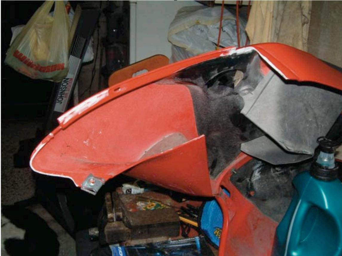
OK, you've done that... now you have to do a similar cut this time to the leading edge of the fairing where it tucks behind the air dam at the front... be sure to leave a tab around the mounting hole where this section screws to the bottom of the air dam.
