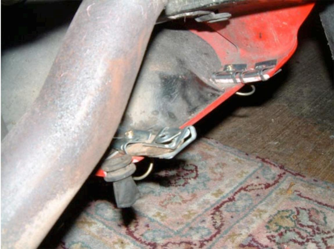
By means of a bit of trial & error, all of the receptacles will need the tab with the locating hole bending in until the pin can lock in place through the fairing... you'll see what I mean when you try it.
