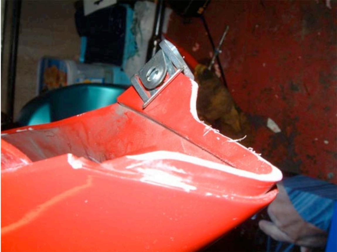
Take the air dam and look at the area where the top fairing screws to the side of the air dam... you need to remove a small amount of fairing to allow the receptacle to slip on over the hole. You can just make out the removed section to the left of the Dzus receptacle..
