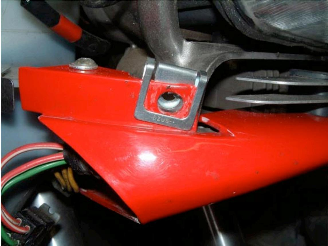
Now to the v-piece... the tab where the two wellnuts fitted will need a small sliver removing to allow the receptacles to fit over the holes. You can see the white bit where the strip has been removed on the right.
