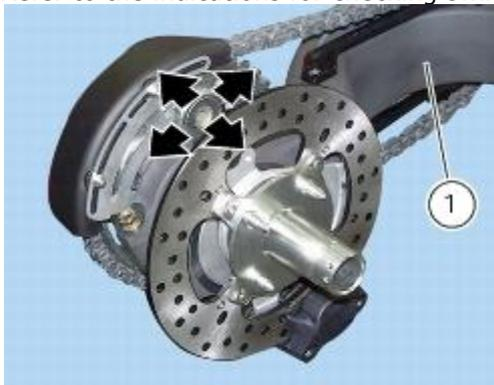
Remove the eccentric rear hub as described in "[Removal of the rear eccentric hub](#)" in this section. Free the speed sensor wiring from the lower chain slider (16) and from the heat shield (22) by unscrewing the bolts (15) and (21).
